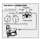
FITTINGS: Install a male plug on the tool which is free flowing and which will release air pressure from the tool when disconnected from the supply source.
