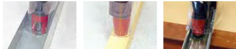
Metal track to concrete
